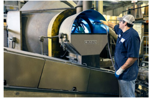
The hinged doors on either side of the vessel provide access to all material contact surfaces for cleaning and visual inspection.
