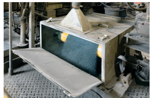
Continuous rotation of the drum during discharge prevents stratification of ingredients having disparate sizes, shapes and bulk densities, and empties the batch in a steady stream.
