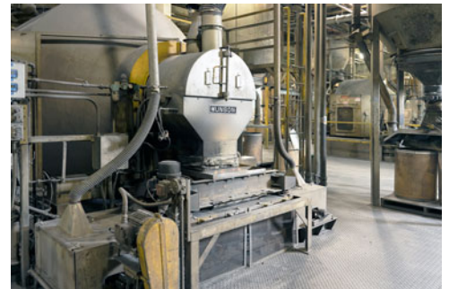
The hinged doors on either side of the vessel provide access to all material contact surfaces for cleaning and visual inspection.
