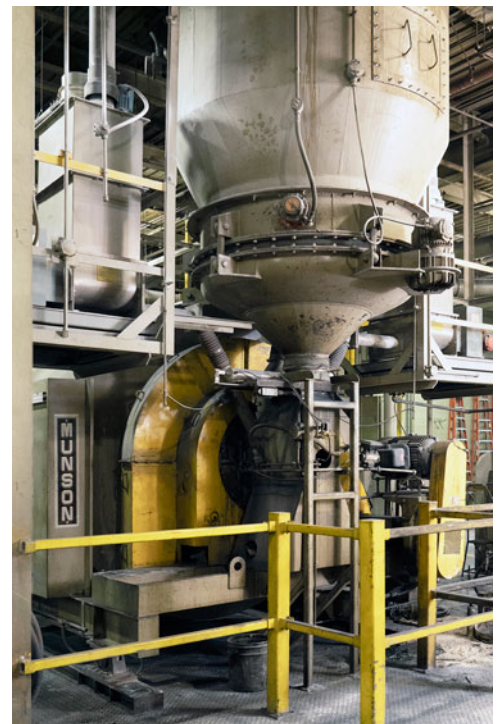
To fill the vessels, a pneumatic conveyor transports resins from compounding units to a holding hopper.
